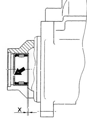
COMPONENT CHECKING AND REPAIR Checking drive-end shield (version with needle bearing) Installing needle bearing: ATTENTION: Heed assembly instructions.
